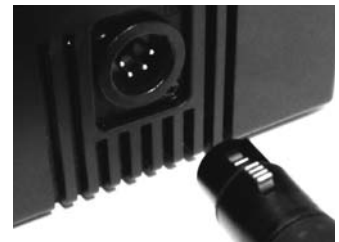
3. Insert 4-pin XLR into 12Vdc Ki Pro power socket
