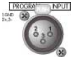
PROGRAM INPUT CONNECTOR XLR-3-31.
