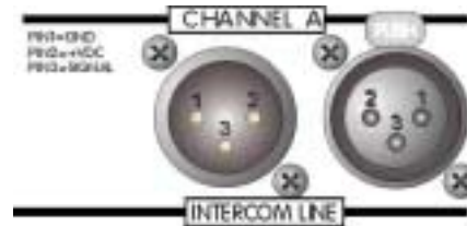
INTERCOM LINE CONNECTORS XLR-3-31 AND XLR-3-32.
