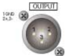
PA OUTPUT CONNECTOR XLR-3-32.
