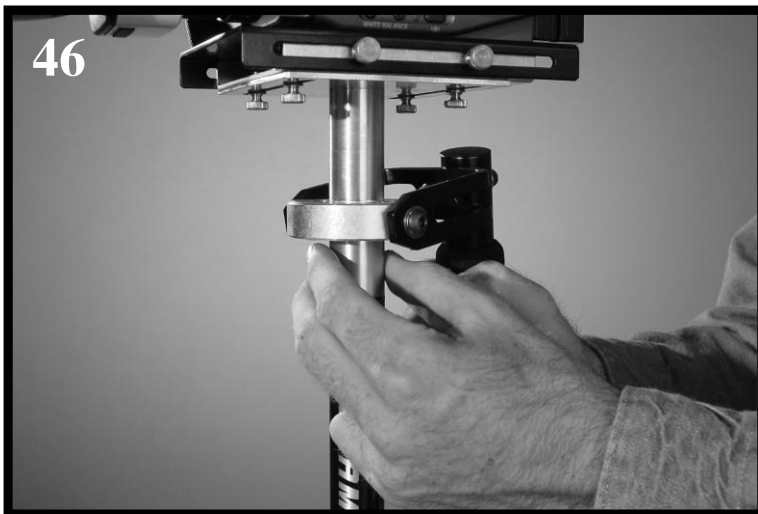
Notice how the “Guiding Hand” does not touch the main bearing assembly or yoke, which can be seen just slightly above the fingers of the “Guiding Hand” in Photo #46.
