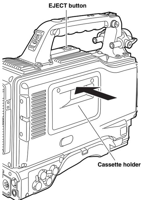
3 Insert the cassette tape and press the part marked with the arrow to close the cassette holder securely.
