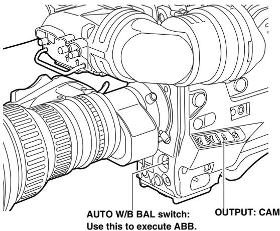
**2** Set the AUTO W/B BAL switch to the ABB position, and then release it.
