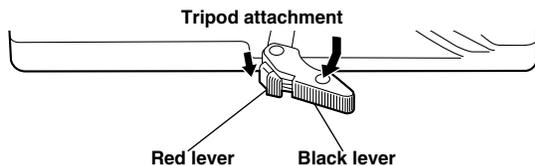
While pushing down the red lever, move the black lever in the direction of the arrow and slide the unit toward the back to remove it.
