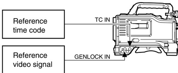
**Example 2:** When connecting a multiple number of units and using one of them as the reference unit
