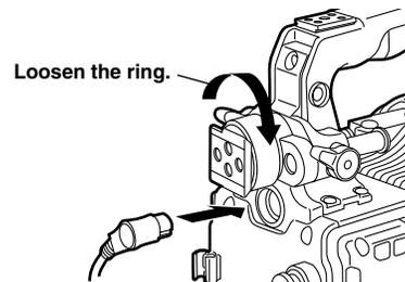
**2** Loosen the viewfinder left-right position anchoring ring.
