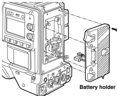
**2** Attach the battery case to the unit.
