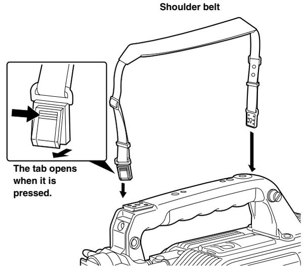
To disengage the shoulder belt, press the tabs.
