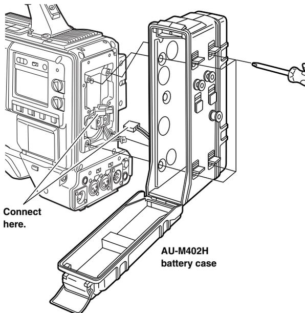
**3** Connect the plug of the battery pack to the connector inside the battery case, and insert the battery pack into the case.
