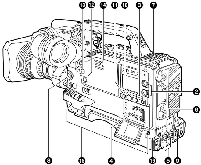
**5 AUDIO IN CH1/CH2 (audio input channel 1 & 2) connectors (XLR, 3-pin)**
