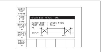
**2** Press the ALT/F2 (FADE TIME) button to select the fade time.
