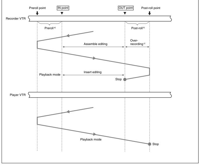
a) Preroll time: Factory-set to 5 seconds. Can be set from 0 to 30 seconds, in units of seconds, through the VTR SETUP menu.
