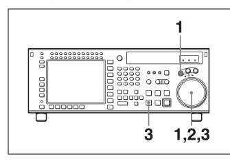
Press the SHUTTLE button, turning it on.
