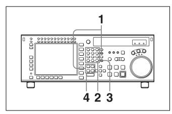
**1** Press one of the IN, OUT, AUDIO IN, or AUDIO OUT button while holding down the RCL button.
