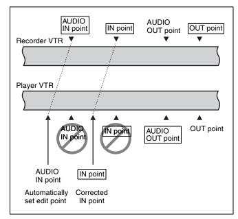
You can use the VTR SETUP menu to select an audio edit mode from among cut, cross-fade, and fade-in/out, and set the duration of the selected edit.
