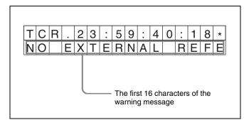
Set the VTR SETUP menu item 626 "DISPLAY INFORMATION select" to any setting other than "time data only" and set the menu item 627 "CHAR WARNING DISPLAY at dual line mode" to "on". The first 16 characters of the warning message flashes on the second line.
