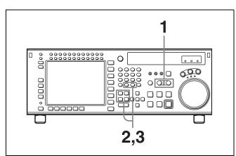
Press the RECORDER or PLAYER button to select the VTR on which to modify the edit point.
