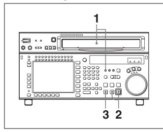
1 Check that the REC INHIBIT indicator is off, then insert a cassette.
