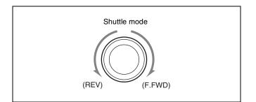
The tape is played back at a speed that corresponds to the angle of the search dial. A direction indicator ( $\blacktriangleleft$  or  $\blacktriangleright$ ) lights up to indicate the direction of playback. The search dial clicks at the positions for still-picture and ±10 times normal-speed playback.
