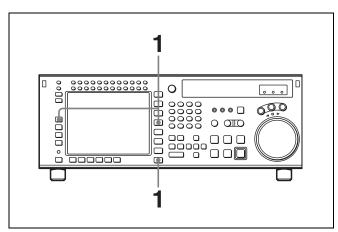
Press the AUDIO button, and in the AUDIO menu press the F1 (AUDIO IN) button, to access the AUDIO INPUT menu.
