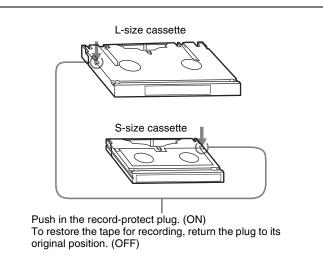
When a cassette with this plug pushed in is inserted into the VTR, the REC INHIBIT indicator on the lower control panel lights up and recording will not start, even if you press the REC/EDIT button.
