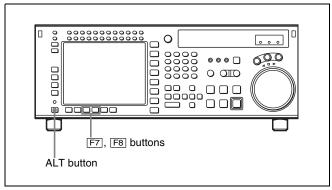
To move in the horizontal direction, press the ALT/ [F7](CHARA H-POS) buttons, and to move in the vertical direction, press the ALT/[F8] (CHARA V-POS) buttons. Each cursor button press increments the setting by 1. From the maximum value, the next value is the minimum value.
