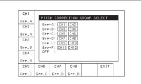
2 Use the F1 (CH1) to F8 (CH8) buttons and the ALT/F1 (CH9) to ALT/F4 (CH12) buttons to group channels (Group-A to F, OFF).
