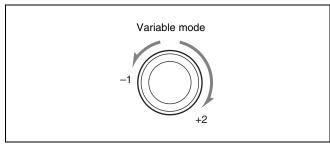
The tape is played back at a speed that corresponds to the angle of the search dial. A direction indicator ( $\blacktriangleleft$  or  $\blacktriangleright$ ) lights up to indicate the direction of playback. The search dial clicks at the positions for still-picture and normal-speed playback.
