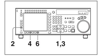
**1** Press the cursor buttons to move the cursor to the cut data to be changed.
