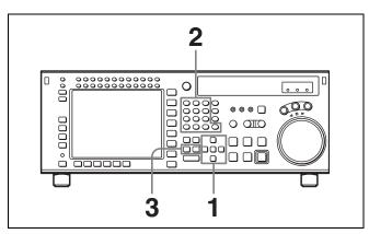
**1** Use the cursor buttons to move the cursor to the IN/ OUT section to be entered or modified.
