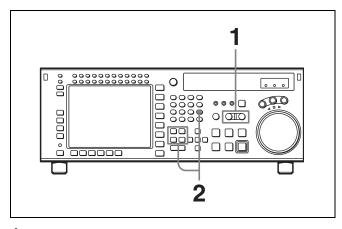
**1** Press the RECORDER or PLAYER button to select the VTR on which to perform the edit point deletion.
