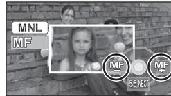
The center of the screen is enlarged. The normal screen returns approximately 2 seconds after you finish bringing the subject into focus.
