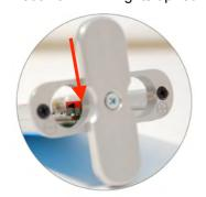
There is a sliding switch inside the battery compartment to change the configuration.
