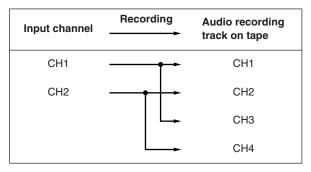
Serial digital multiplex signal input (SDI: option) (Setup menu item No.712 setting: CH1/CH2)
