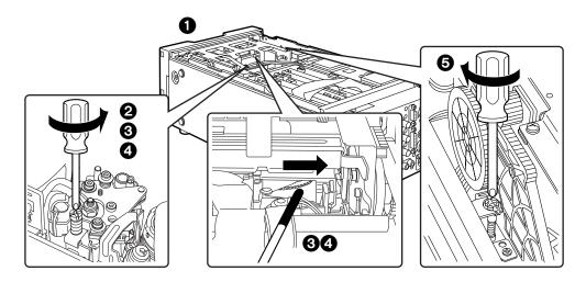
This unit is equipped with an auto head cleaning function, which automatically reduces the amount of dirt on the video heads. However, in order to enhance the unit's reliability, it is recommended that the video heads be cleaned every day. Use a cleaning fluid designated by the unit's manufacturer.
