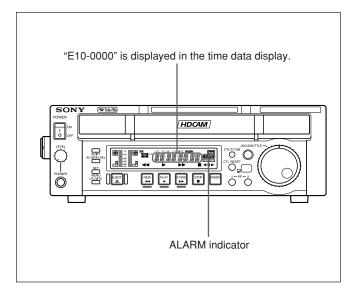
If this happens, the drum and capstan motors stop and the cassette is automatically ejected. Then, the drum starts to rotate again to dry its surface. In this state, the unit is not operable. When the moisture has evaporated, the ALARM indicator goes off and the "E10-0000" message disappears.
