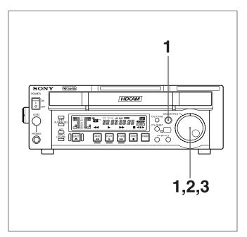
In jog mode, the JOG dial controls the playback speed based the speed at which the dial is turned. The playback speed range is ±1 times normal speed. Use the following procedure to carry out playback in shuttle mode.
