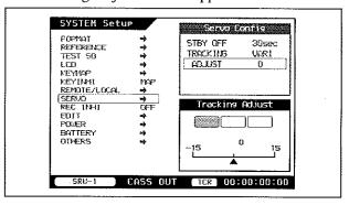
While viewing the channel condition display, rotate the ADJUST knob or SELECT/ENTER dial to adjust so that the channel condition display lights in green.
