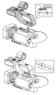
④ Press and turn the handle mounting screws to tighten them.
