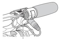
Put the cable in the outer cable holder.
