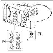
You can adjust and fix the white balance according to the lighting conditions of recording environment.
