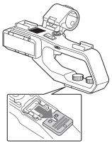
③ Align the mark on the XLR handle with the one on the camcorder, and insert the XLR handle unit in the direction of the arrow.
